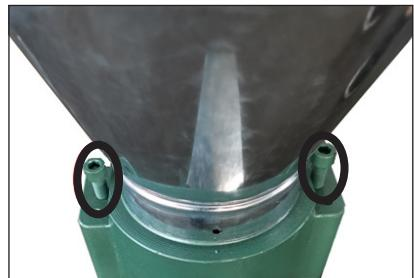
**NOTE !:** The screws should be identically tightened. If they are tightened too much, one of the rollers may stop turning and / or the roller may become deformed. Also, do not increase the pressure of the rollers by tightening the screws in the event that the die is clogged.
