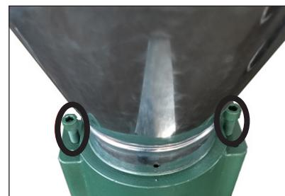
**NOTE !: The screws should be identically tightened. If they are tightened too much, one of the rollers may stop turning and / or the roller may become deformed. Also, do not increase the pressure of the rollers by tightening the screws in the event that the die is clogged.**
