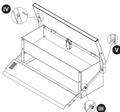
Tip! To help the birds get used to the feeder and learn how it works, it is recommended to tighten the screws from the higher hole to the lower one.
