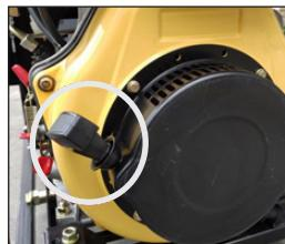
4. press the pressure reduction lever (after removing the starter, it will automatically return to its original position)
