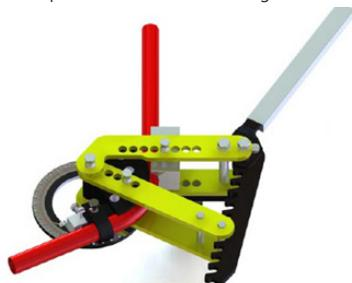
Caution: When bending a pipe above 120 °, a pipe may get stuck in the machine. Then, to release the pipe, first remove the pin blocking the strap and then gently tap the pipe. This will make it easier to remove.
