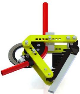
3. Remove pin 7/8 ". Turn the swivel arm counterclockwise (being careful not to move the pipe). Insert 7/8 " pin and repeat the bending process until the desired angle is achieved.
