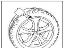
**WARNING:** Not lubricating the rim bead will cause serious damage to the tyre.
