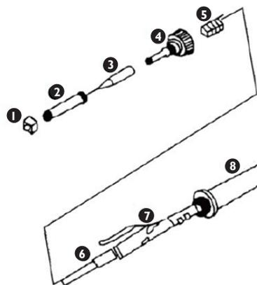
1. nut for mounting the soldering iron tip housing
