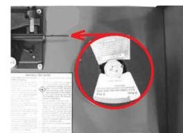
After installing the wire spindle, fit the upper fixing plate, spring and knob.
