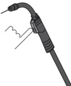
Press the button on the welding clamp (the tip of the welding clamp should be as far away as possible from any object) and pull out about 5 cm of the welding wire.
