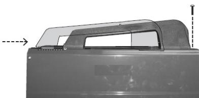
Insert the handle into the fixing holes in the upper cover and secure with a bolt.
