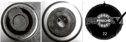
c) The seal of the type shown below has a safety pin which needs to be removed (No. 23 has three pieces and No. 24 has two pieces). To remove the safety catch, gently pull on the safety catch and then invert it and pull it out of the barrel. In its place, place the gasket supplied with the beer tap, which should be pierced with a pin when installing the keg to the tap
