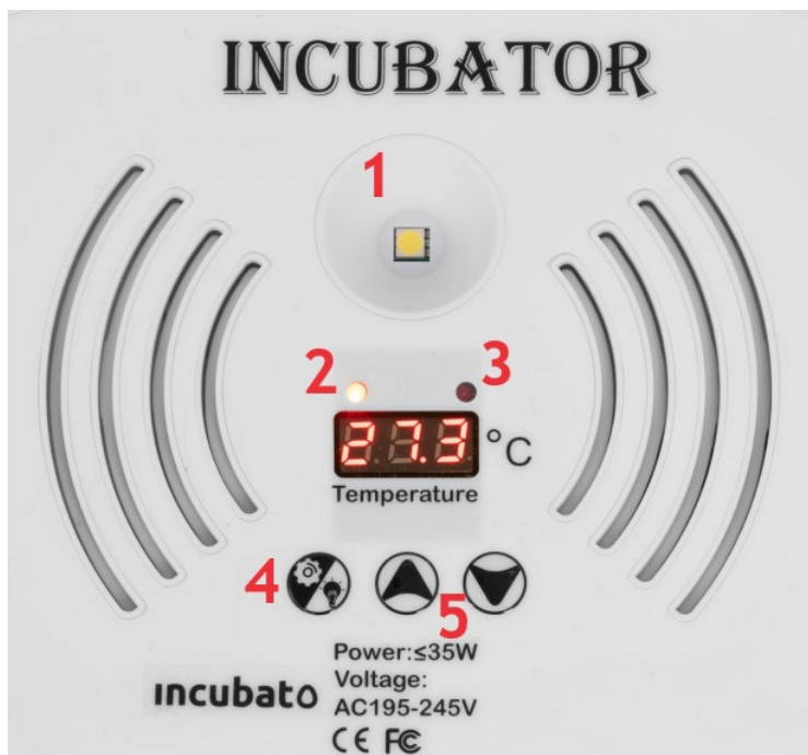
1 – Ovoscope / 2 – Operating (heating) indicator light / 3 – Parameter setting indicator light / 4 – Temperature setting button (press once) / Ovoscope switch (to turn on press for 3 seconds. To turn off press again, if not pressed then the light will turn off after 6 minutes) / 5 – Buttons for increasing / decreasing the temperature value. Button for decreasing temperature value is also the button for test eggs turning (long press).
