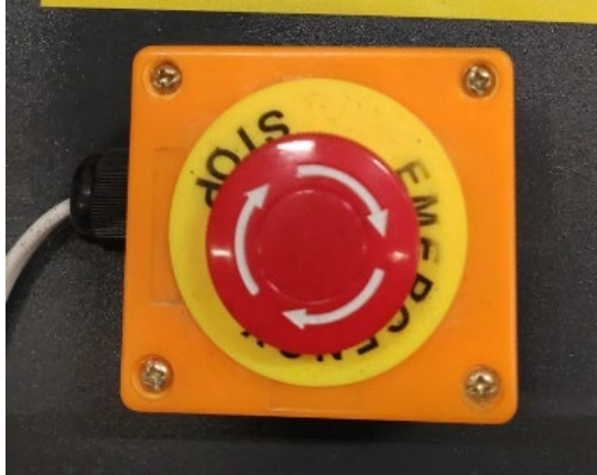
EMERGENCY STOP (red mushroom) - emergency stop button of the machine.
