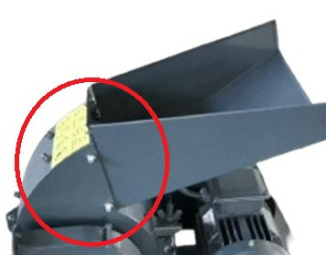
Fix the inlet chute of the raw material to be processed
