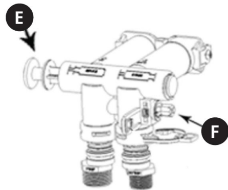
Position for softened water supply
