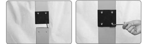
2. Connect the two wires, then insert the lower end of the column into the rectangular hole in the base. Tighten the 2 M6x20 screws with an Allen key.
