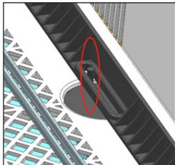
3. Plug the power cord into the socket on the device.
