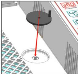
2. Make sure that the protruding part of the shaft fits into the handle of the egg tray.
