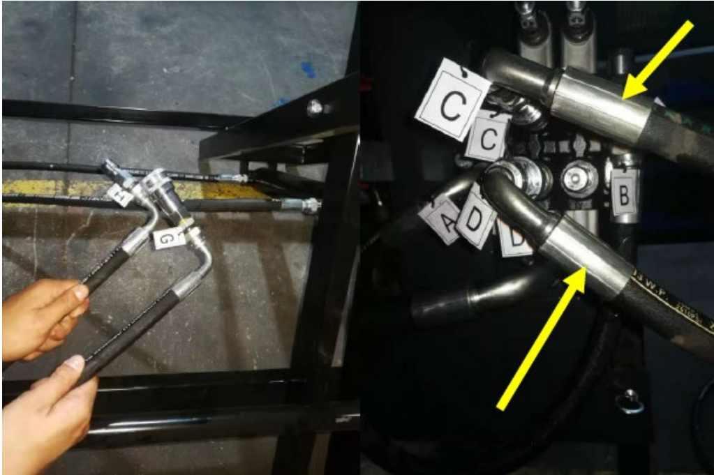
H/G – log lifter cylinder connection for the lifter motor.
