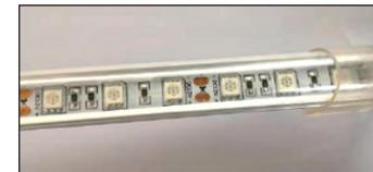
2. Connect the lamps in series so that the last terminal module is without an output wire.
