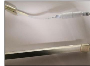
3. Connect the male end from the power supply to the female input of the first lamp. Optionally, when using remote control for lamp control, connect a controller module between the male end of the power supply and the female end of the lamp.
