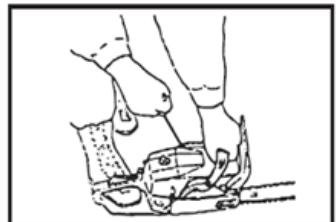
Before each use, check if the brake is working properly:
