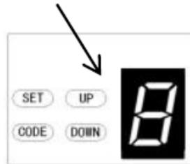
b) Press the **SET** button again, the unit is now in partial open/height adjustment mode. And then you will see a figure “0” with flash dot appears on the display.
