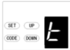
d) Press **SET** button to confirm the set and it will be back to standby status automatically and display “11”.
