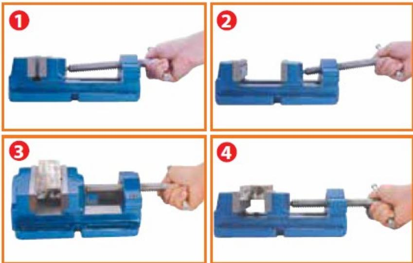
**CAUTION:** in order to ensure long and problem free operation of the device, the fixed element should be located in the middle of the jaws, if possible. Vices also have grooves in the jaws for a more secure grip of round items.
