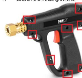
2. Remove the top of the housing and route the welder cable through the gun: route one end of the cable to the trigger and the other end through the head to the handle.
