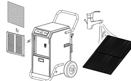
**CAUTION!** Do not use the device without the air filter – it may pollute the evaporator! Do not touch the evaporator surface with bare hands – the risk of injury!
