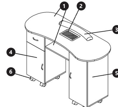
1. Counter with a hole and a shelf for a dust absorber
