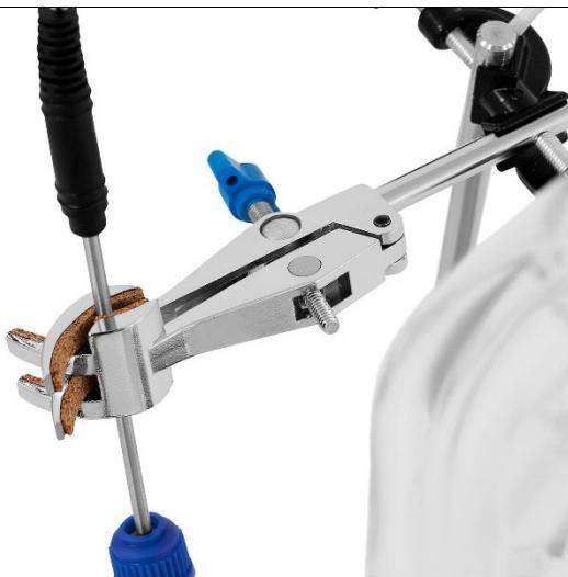
8. Withdraw the internal thermocouple (if connected) from the socket in the base of the heating jacket.
