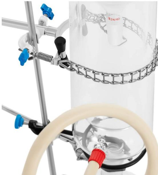
26. Secure the connection between the chiller [17] and receiving flask (1000 ml) [20] with a clip.
