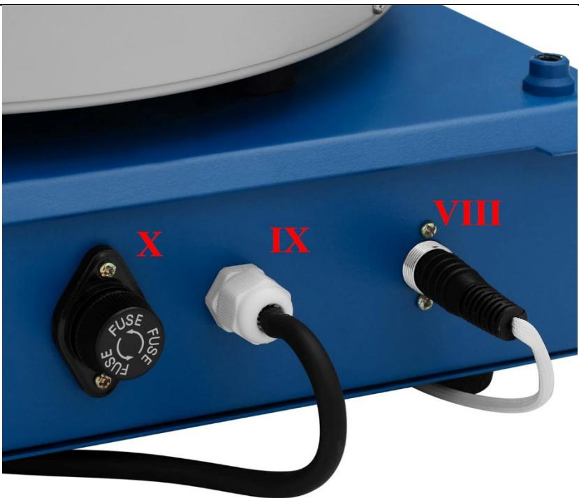
VIII - external/internal thermocouple socket
