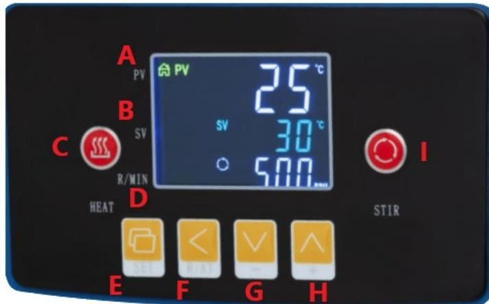
A - PV - measured (current) temperature value
