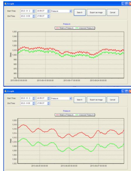
With the "Export as image" button, you can export the selected graph into a .jpeg format file. You can change the Y axis by scrolling the mouse up and down roller.
