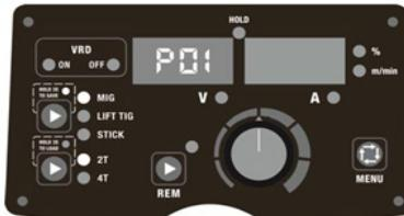
Fig. 15. Saving parameters at the address P01
