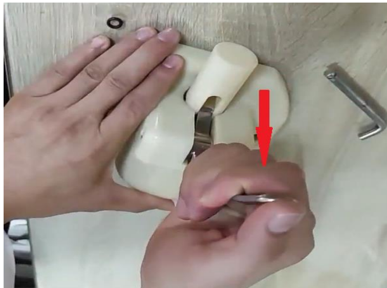
3. Pull the Lever down and remove it
