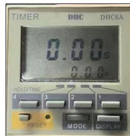
In a given setting, the most important are the „4, 3, 2, 1“ buttons, which allow you to set the exact time of one filling cycle from the range of 00.00-99.99 seconds - each button is subordinate to a given digit, and each time it is pressed, its value changes in the range of 0-9. After each cycle, the device stops automatically and enters the standby mode.
