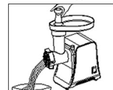
Assembling the device with a butcher's overlay.
