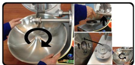
Open the dish cover, then turn the dish clockwise at an angle until it feels loose. Then lift it up a little and pull it out. When refitting it, make sure that it snaps into the mount by turning it counter clockwise until it cannot be turned any further.
