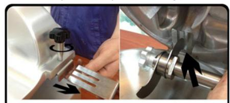
Unscrew the knob which secures the locking partition, then pull the partition out. When attaching it, make sure that the partition is tilted downward and that it is fully inserted. Then fix it in place with the knob. When you have finished, make sure that the knife blade passes smoothly through the slots in the partition - i.e. nothing grinds against it or blocks it.
